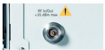
**RF IN/OUT** is a 50  $\Omega$  N-type connector (female) on the left-hand side of the rear panel.
