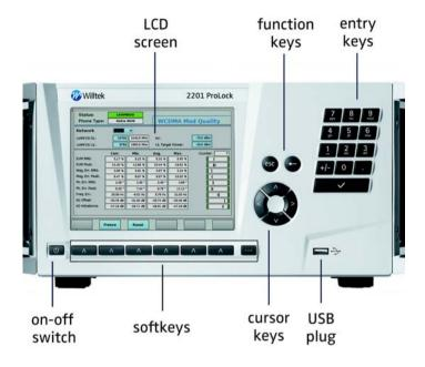
**LCD** The LCD screen shows the menus that guide you through configuration and measurements when the 2201 ProLock is switched on and the operating software is loaded. The menus consist of different sections as follows:
